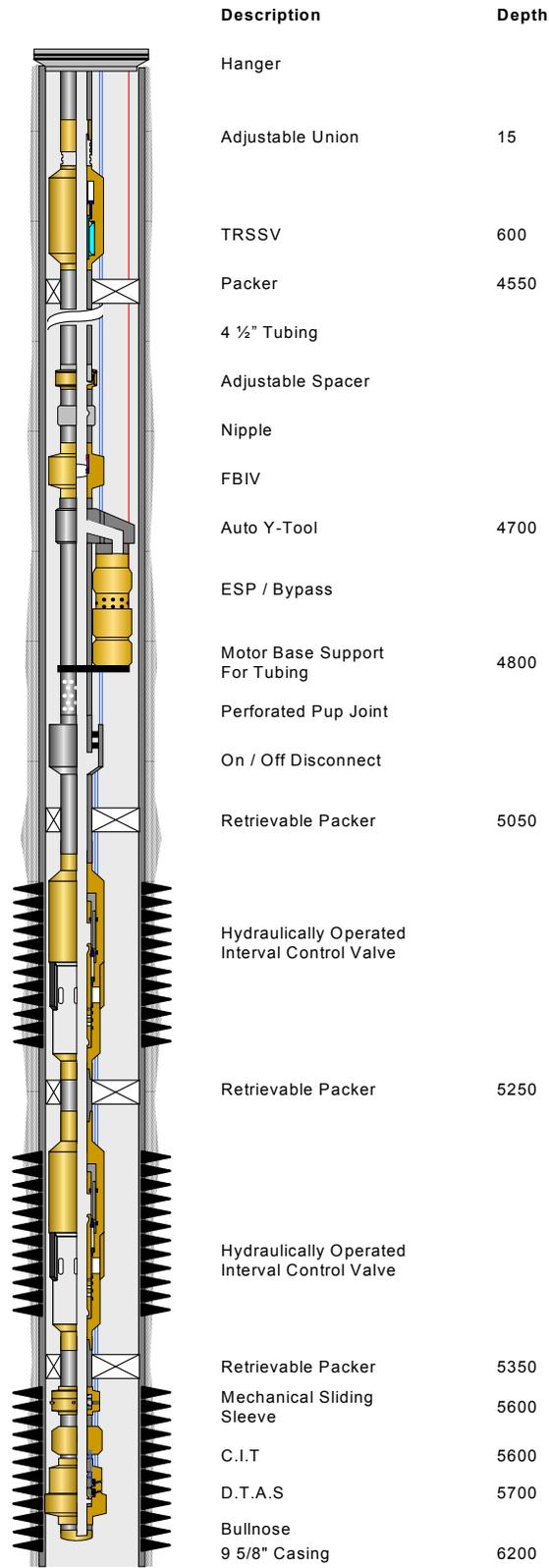
Fig. 5 — The D17 Multizone Completion
