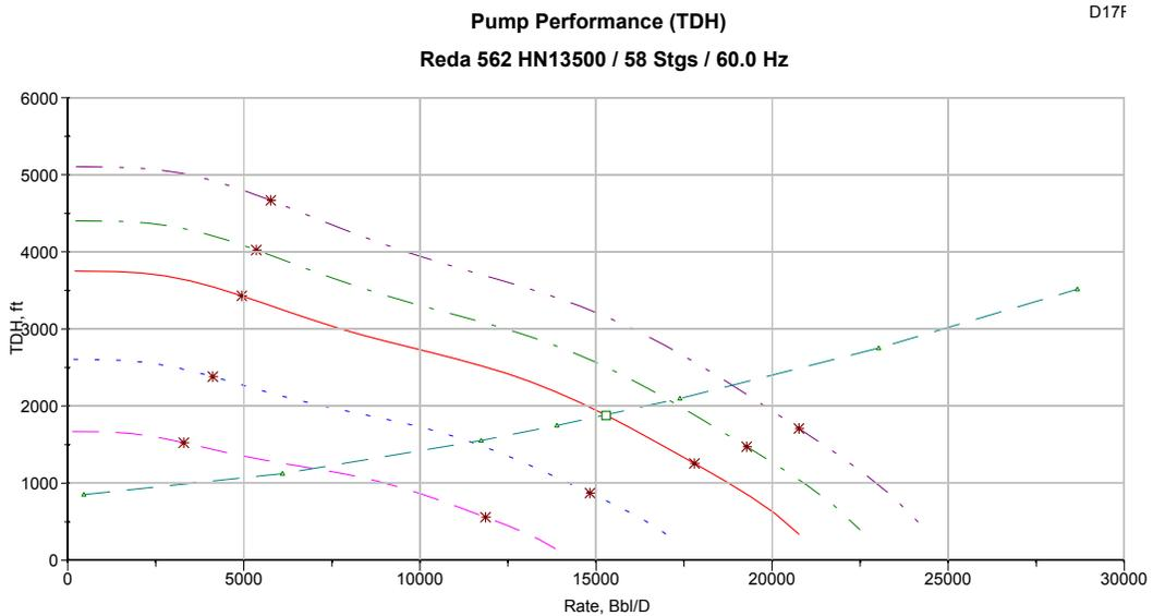
Fig. 7 — Lift Curves and Inflow Performance of the Well Before Closure
