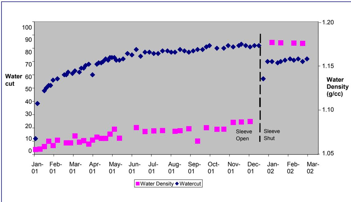
Fig. 9 — Performance of Well Before and After the Closure of the Interval Control Valve
