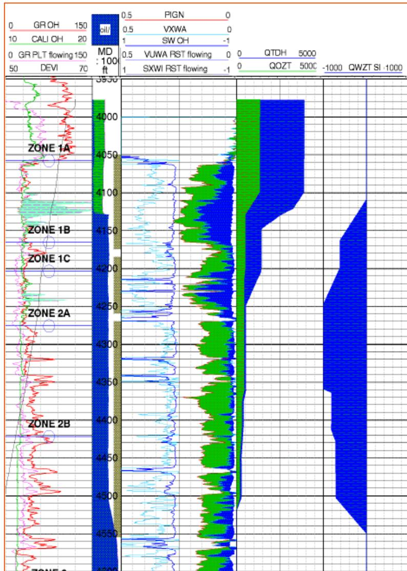
Fig. 4 — Representative Production Log Showing Water Entry Locations.
