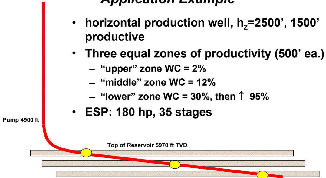
Fig. 1 — Hypothetical Horizontal Production Well That Penetrates 3 Layers.
