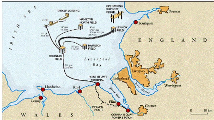
BHP's Liverpool Bay development incorporates drilling and production facilities, a mobile support vessel, oil storage barge, subsea pipelines, gas terminal and export gas pipeline, and onshore base — all in the full view of the local community.
