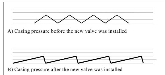
Fig. 3 Casing pressure behavior before and after the installation of the new pilot valve in well A
