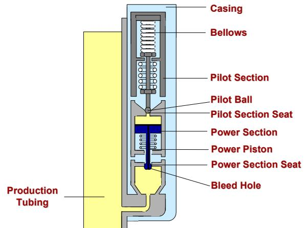
Fig. 1 Pilot valve main components
