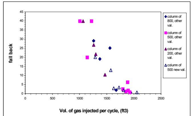
Fig. 2 Fall back losses vs. volume of gas injected per cycle.
