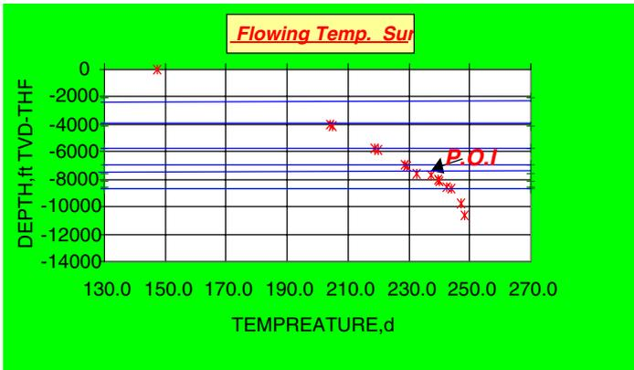
Fig (3) Temperature profile for Gas lift well.
