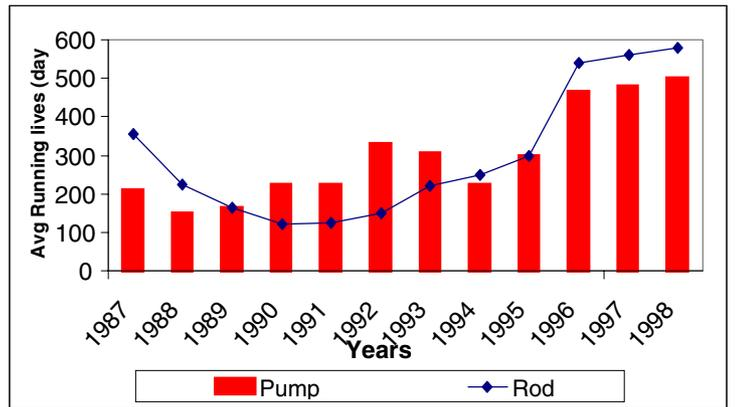
Fig. (7) Avg Running lives for rods and pumps for Agiba case study.
