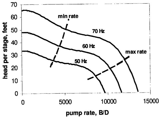
Fig. 2 – Typical pump curve. The region between low and high frequencies and the minimum and maximum recommended rates is called the “pump tornado”.
