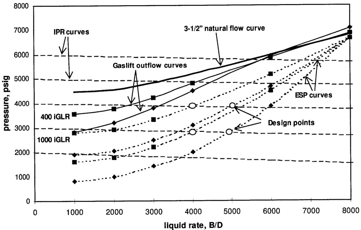
Fig. 9 – System curves for natural flow, gaslift and ESP
