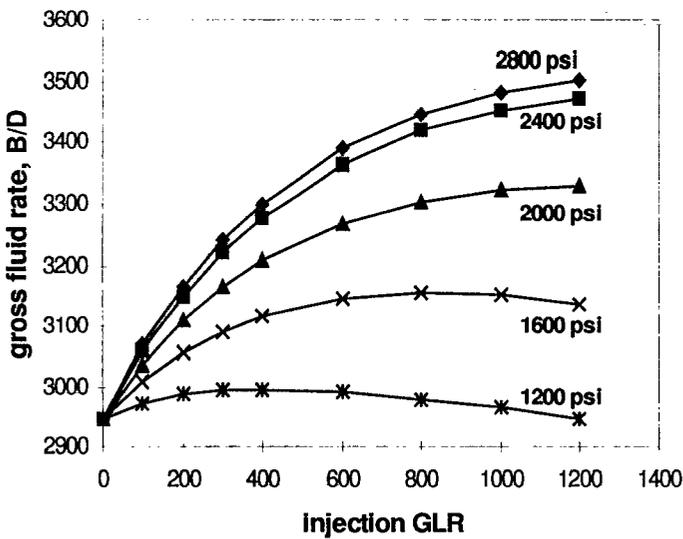
Fig. 5 – Gaslift performance curve for mid-life depletion case
