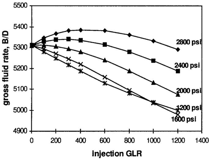
Fig. 4 – Gaslift performance curve for early life depletion case
