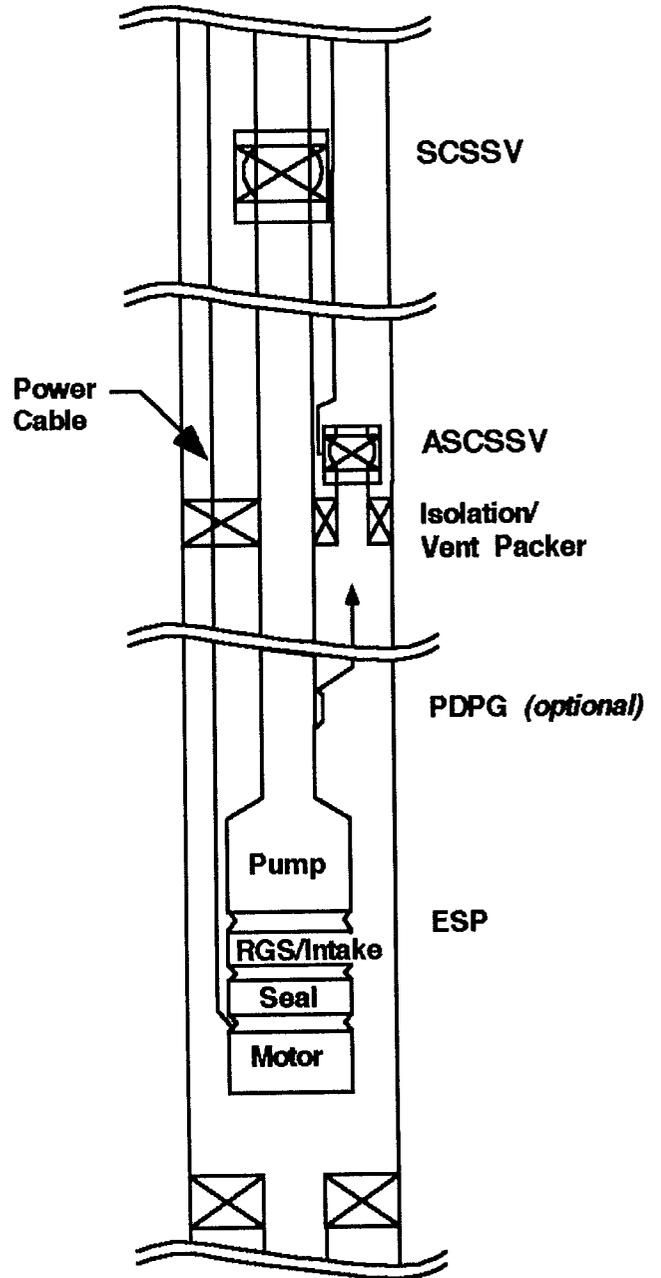
Fig. 3 – ESP with gas separator, packer and annular SCSSV.
