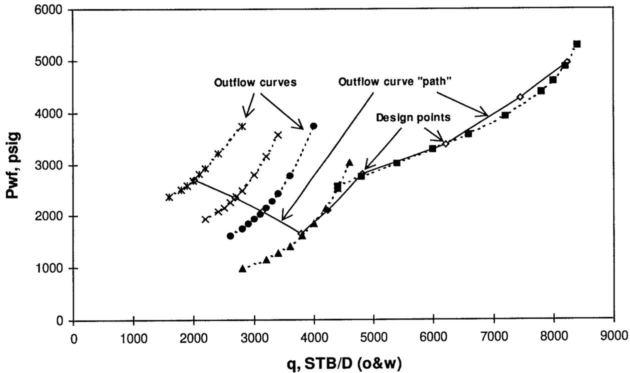
Fig. 8 – Outflow curves for ESP, showing individual design points and outflow curve "path".
