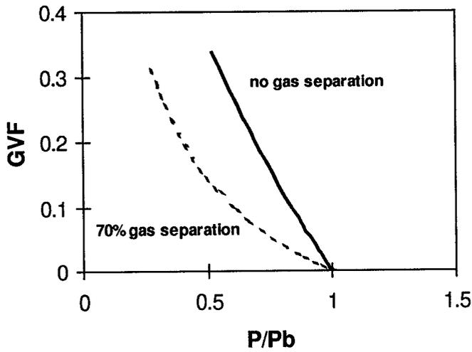
Fig.1 – Gas volume fraction as a function of pressure below bubble point. The impact of gas separation at the intake is shown.
