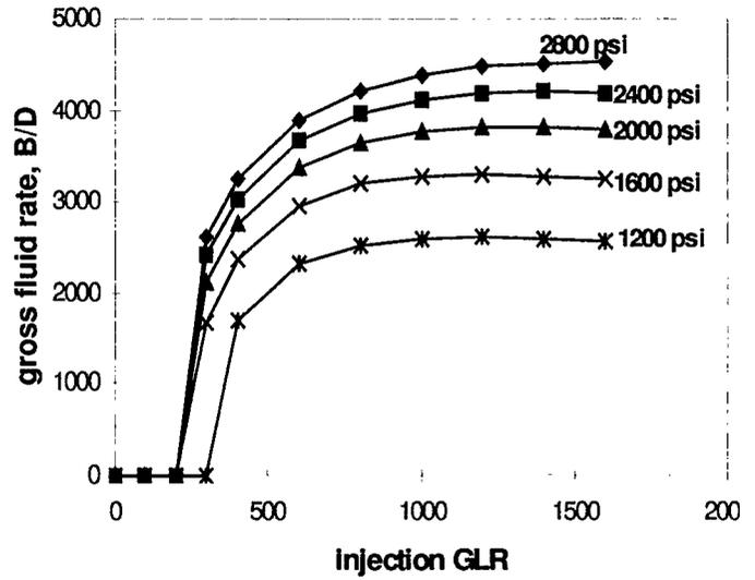
Fig. 6 – Gaslift performance curve for late-life waterflood case.
