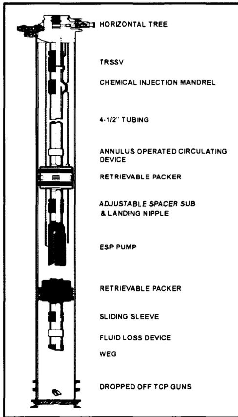
Figure 4 Douglas ESP Completion Schematic
