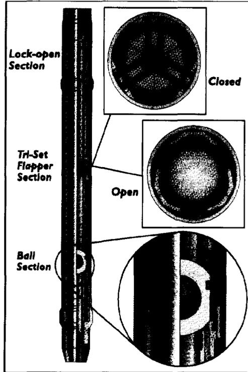
Figure 6 Fluid Loss Device
