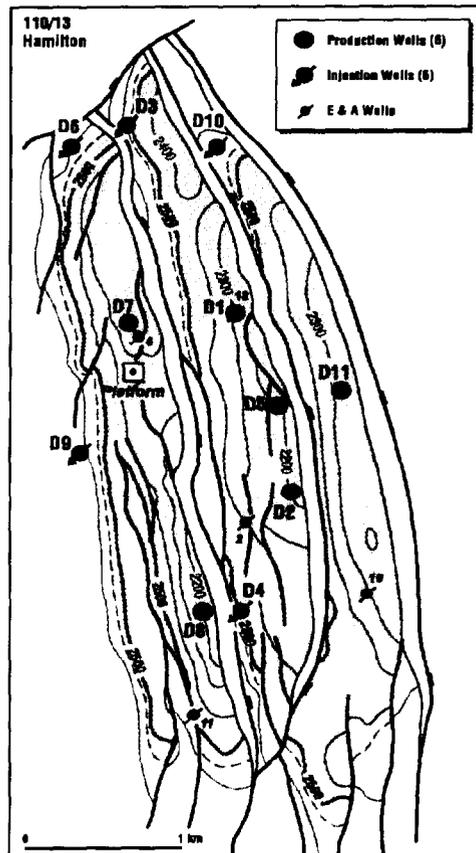
Figure 2 Douglas Reservoir Top Structure
