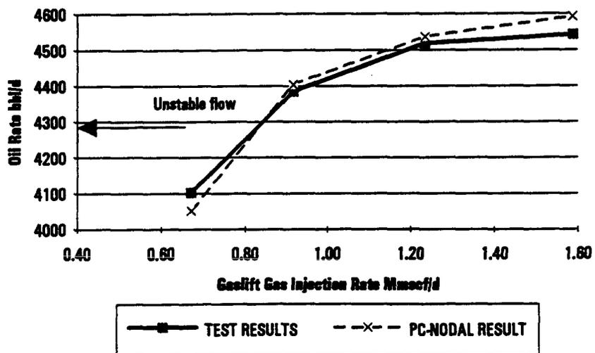
Comparison of Test versus Computer Model
