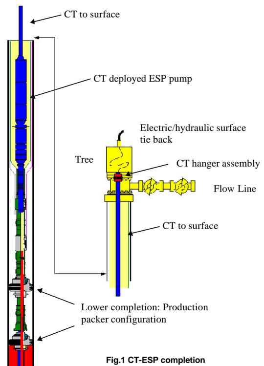
Fig.1 CT-ESP completion
