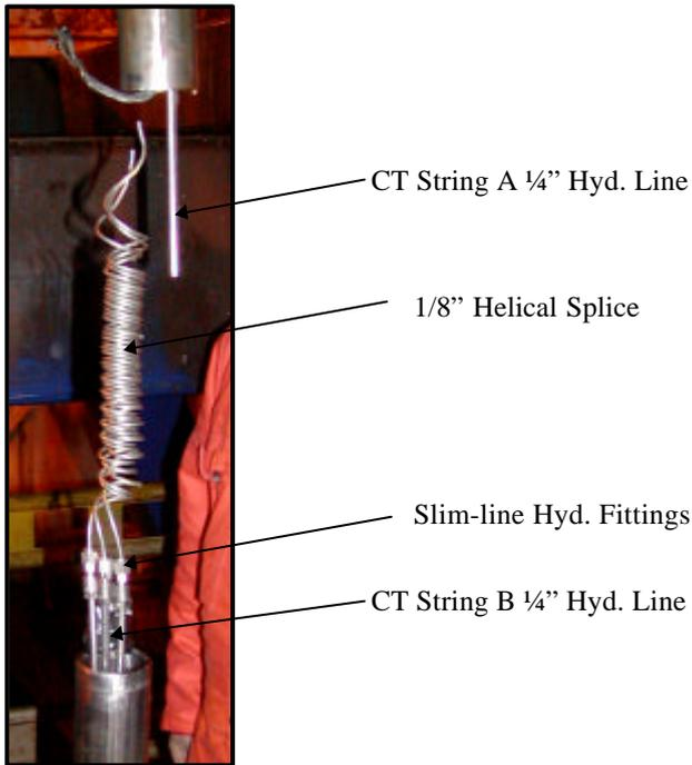
Fig.11 Splicing Procedure
