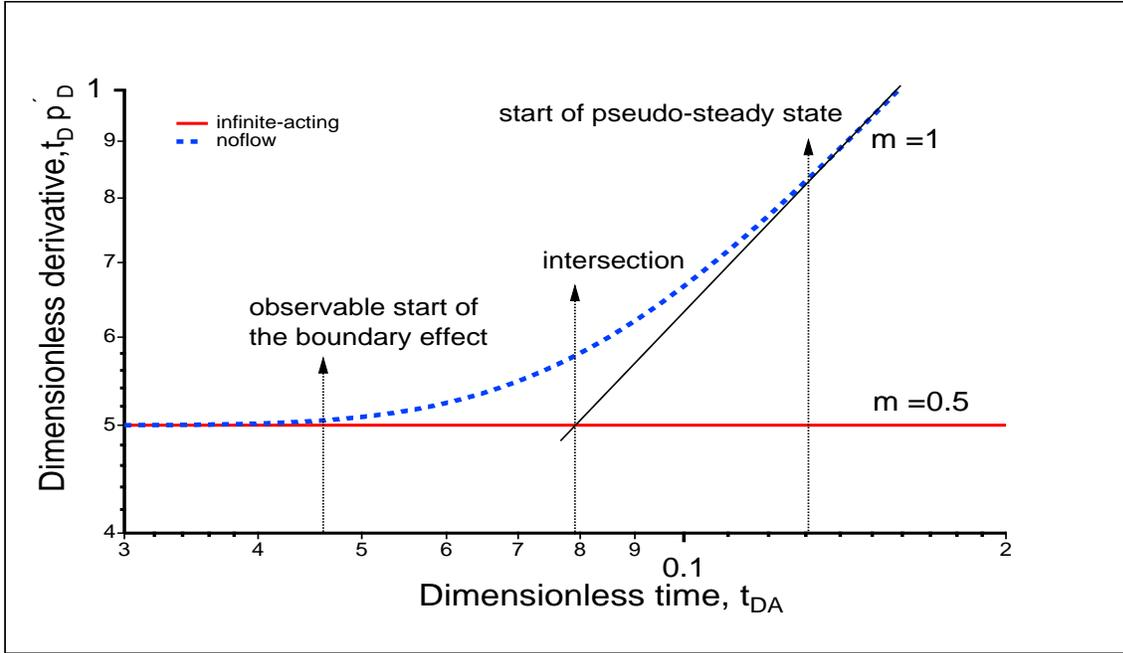
Fig. 8—Dimensionless pressure derivatives for infinite-acting and no-flow outer boundary systems as a function of dimensionless time  $t_{DA}$ .
