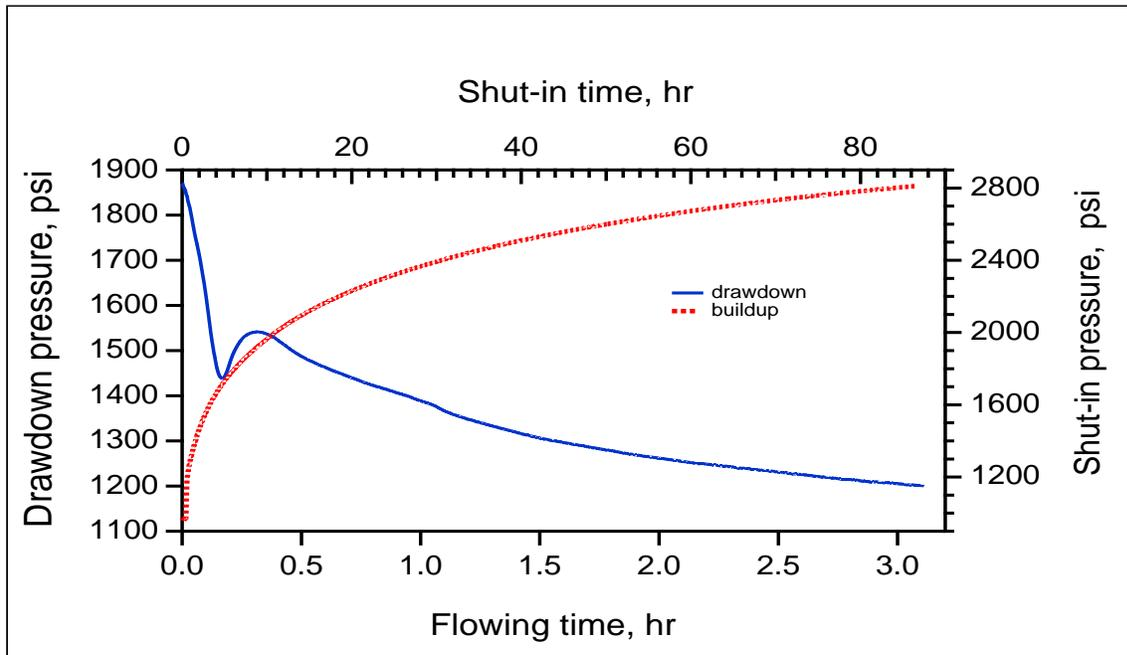
Fig. 10—Wellbore pressures for a drawdown and a subsequent buildup test.
