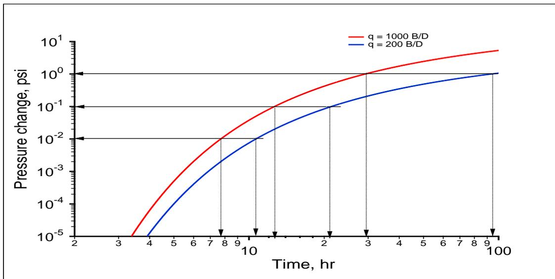
Fig. 3—Additional pressures changes at the wellbore due to a sealing fault.
