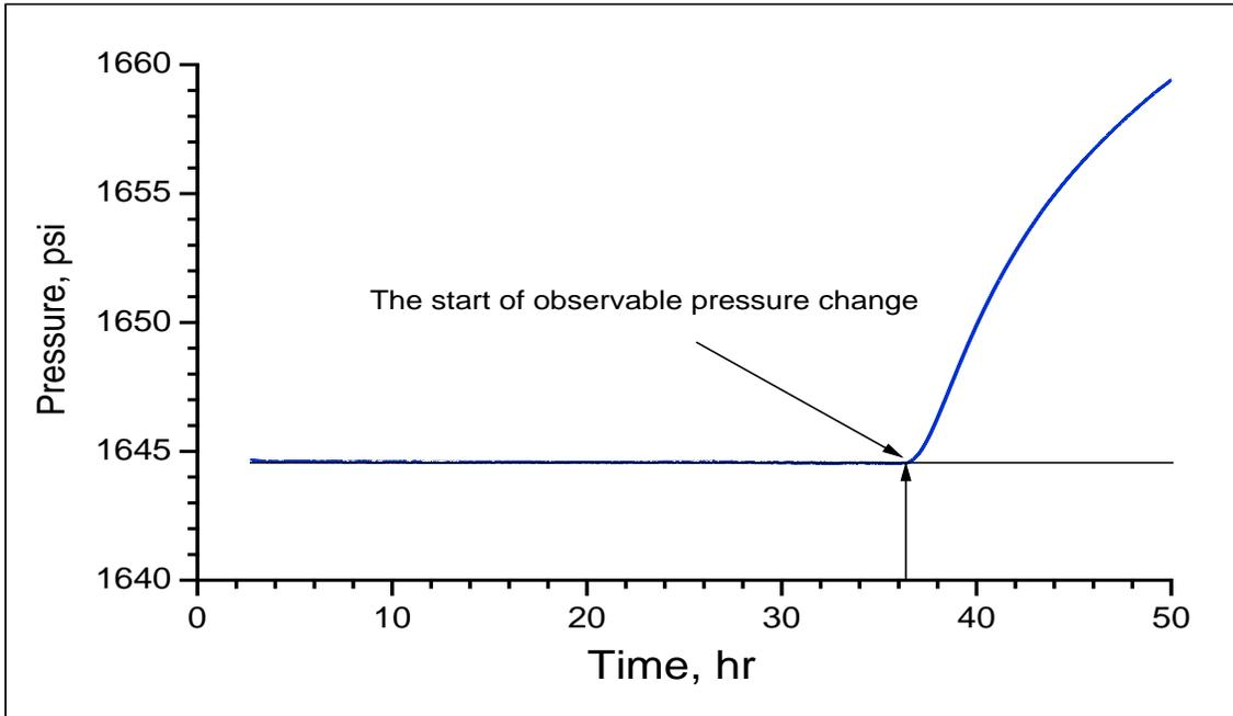
Fig. 1—Pressures response at an observation well due to an injector.
