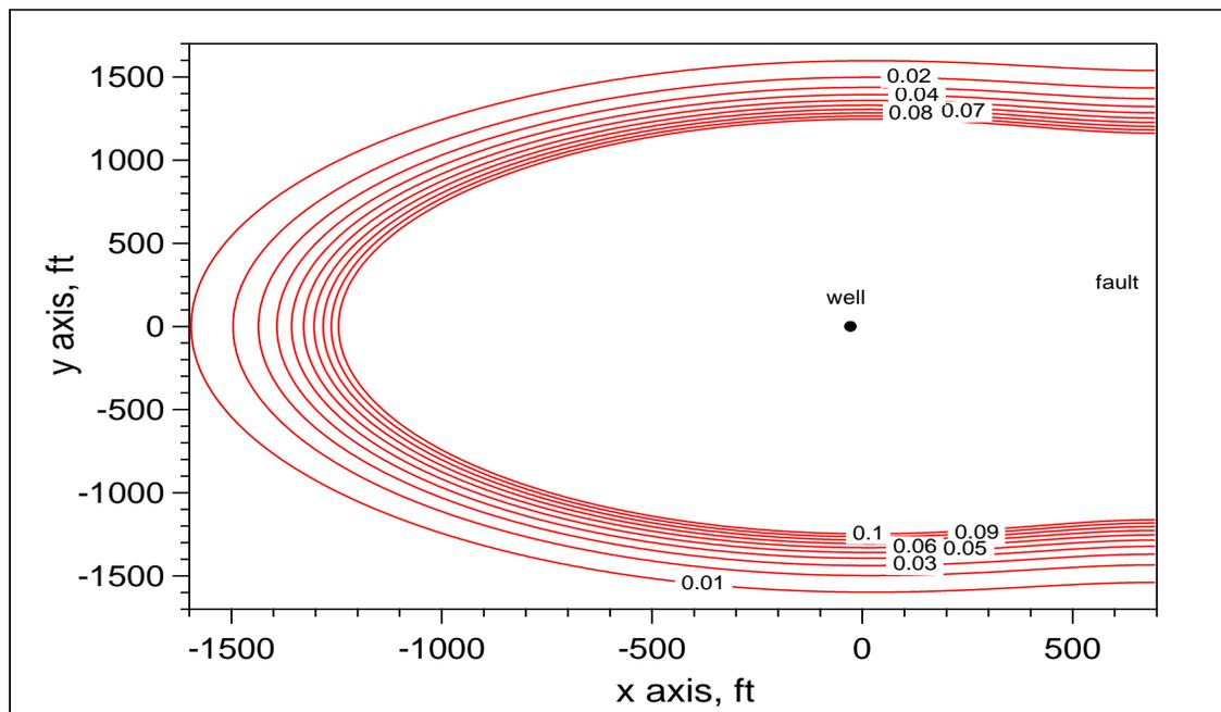
Fig. 14—Pressure distribution in the reservoir for the sealing fault example.
