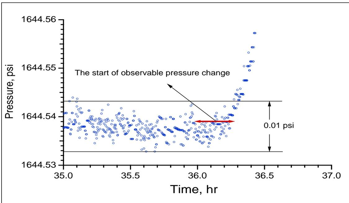
Fig. 2—Pressures response at an observation well due to for an injector.
