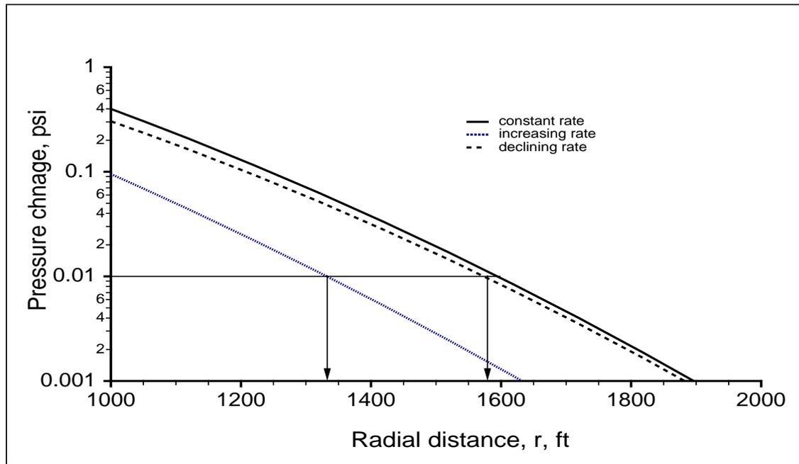
Fig. 13—Reservoir pressure distributions for linearly declining and increasing flow rate cases.
