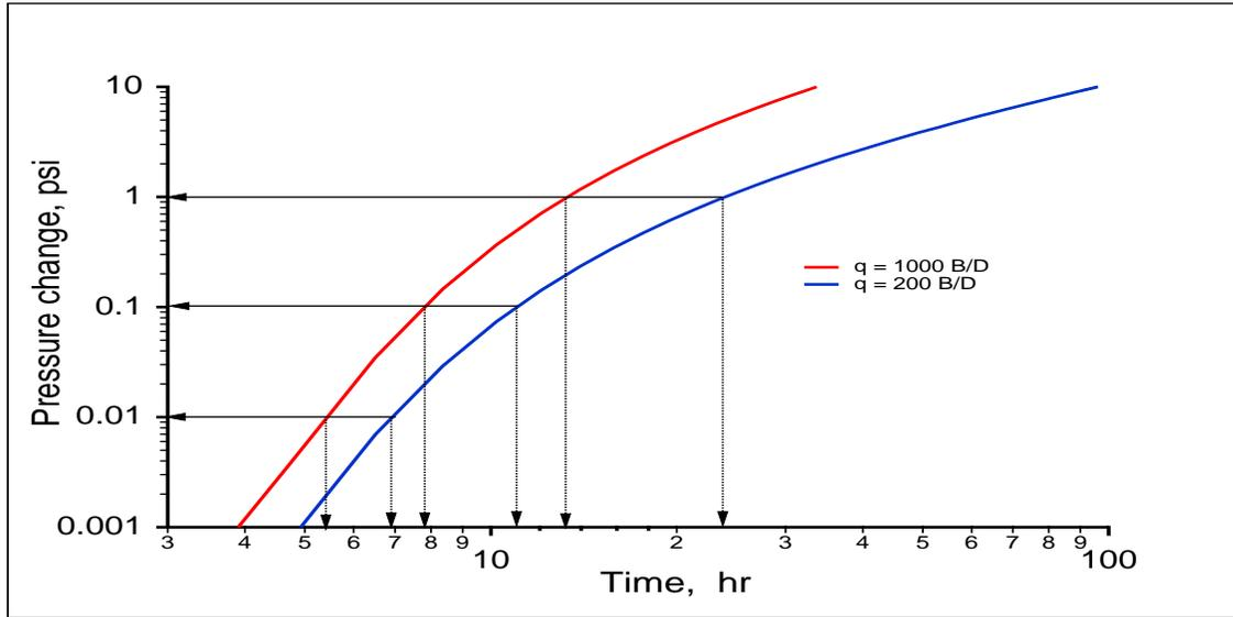
Fig. 6—Additional pressures change at the wellbore in a closed no-flow reservoir.
