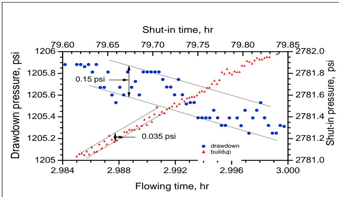
Fig. 11—A time period showing wellbore pressures for a drawdown and a subsequent buildup test given in Fig 10.
