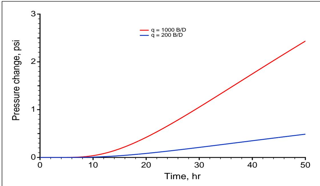
Fig. 4—Additional pressures changes at the wellbore due to a sealing fault.
