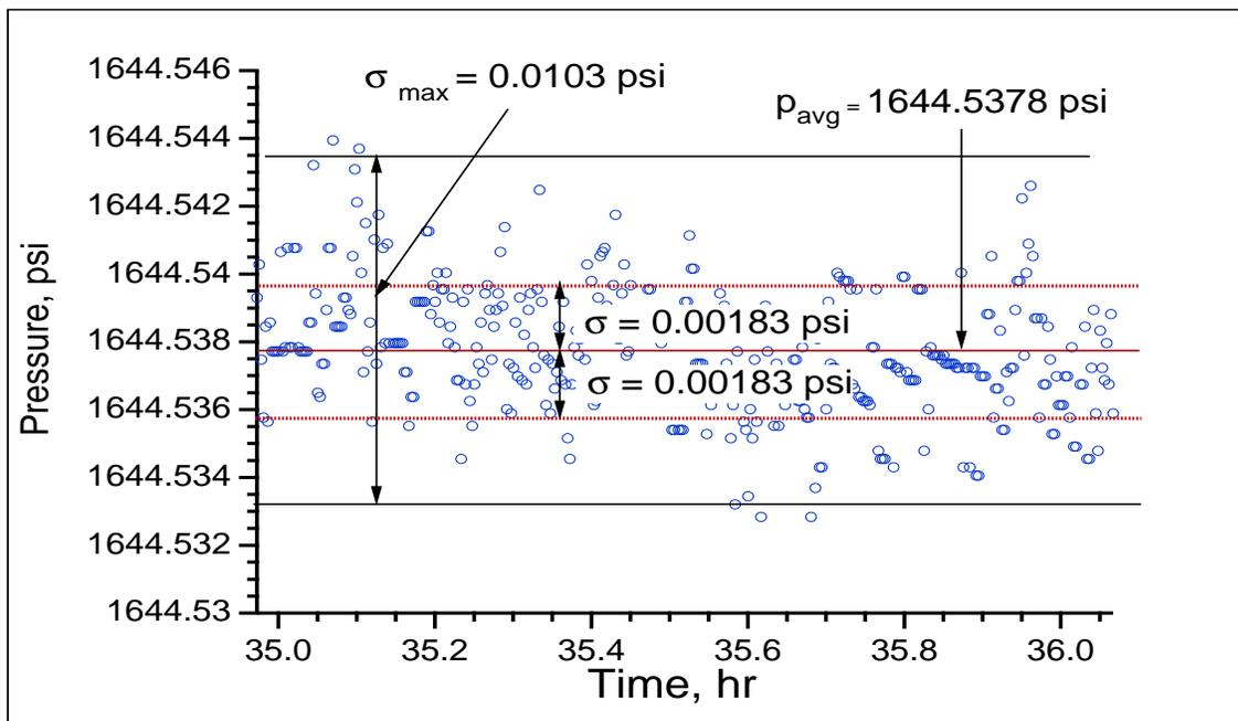
Fig. 15—Determination of an apparent resolution from an interference test data.
