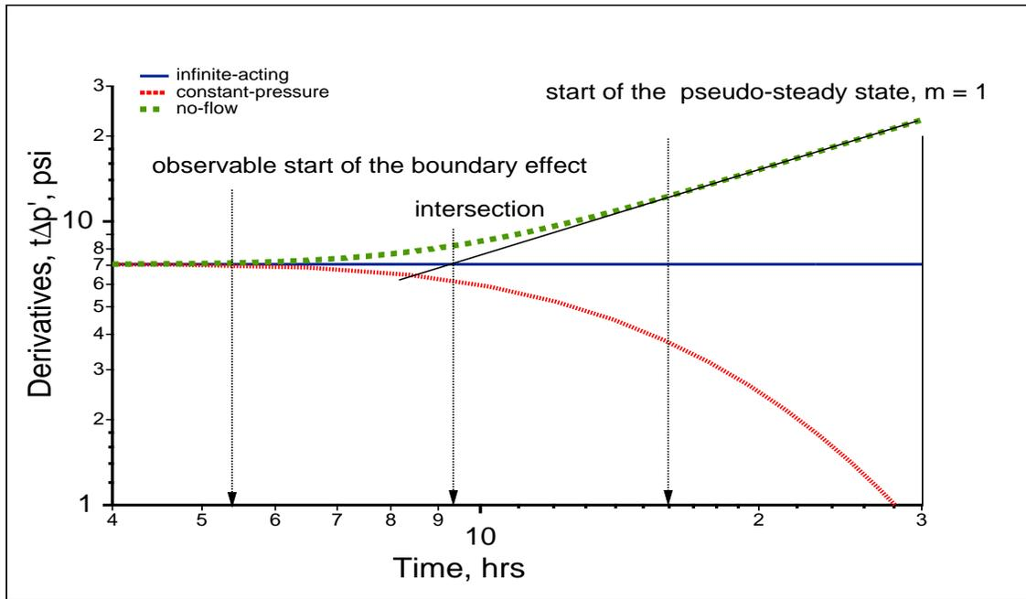
Fig. 7—Derivatives of the wellbore pressures for an infinite-acting system, and a no-flow and constant-pressure outer boundary systems.
