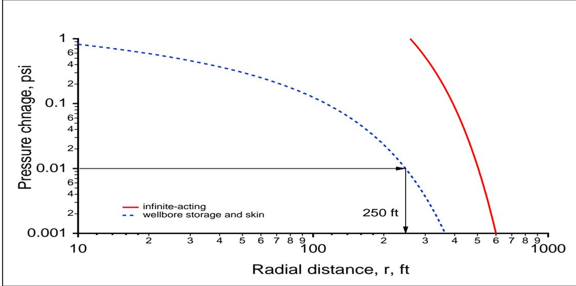
Fig. 12—Reservoir pressure distribution with and without wellbore storage and skin effects.
