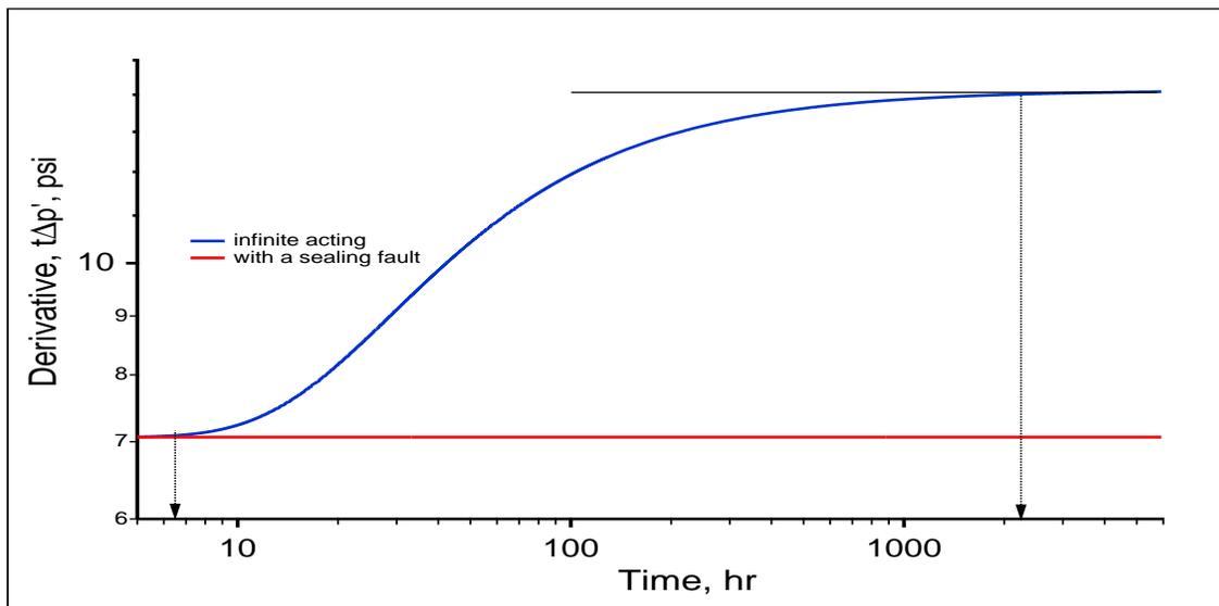
Fig. 5—Derivatives of the wellbore pressures for an infinite-acting system and a reservoir with a sealing fault.
