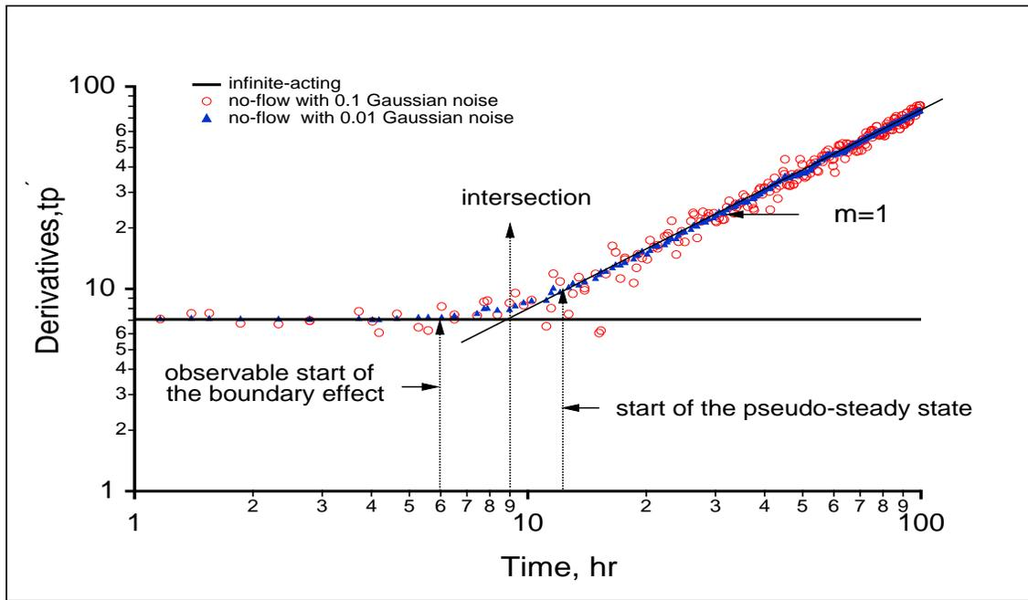
**Fig. 9—Derivatives of the wellbore pressures with noise for an infinite-acting system and a no-flow outer boundary system.**
